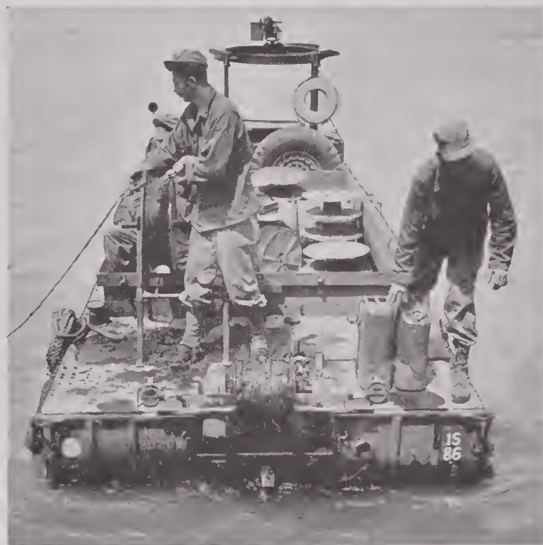
FIGURE 35. DUKW used by Signal Corps for laying underwater communications in Admiralty Islands.
